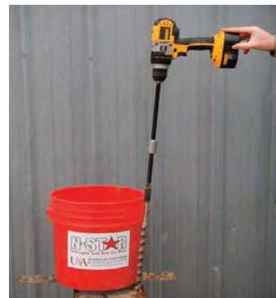
Photo 9-1. N-STaR soil sample bucket, soil auger and drill.
