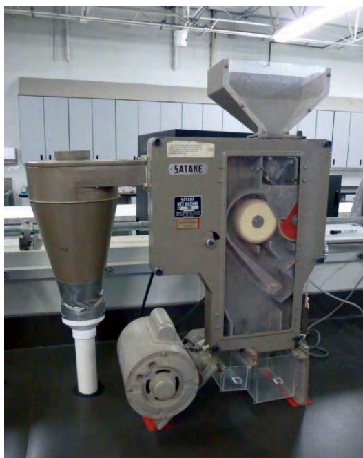
Photo 14-1. A laboratory-scale rice huller (THU 35B, Satake, Hiroshima, Japan).
