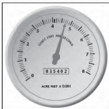
Dial with cubic feet per second indicator and acre-ft totalizer. Place a decimal point three places to the left. Acre-ft = 835.402
