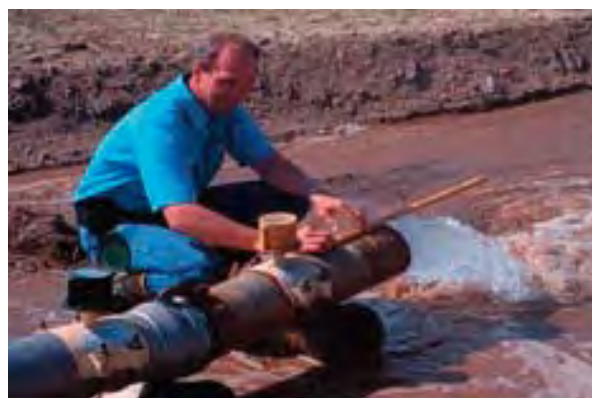
Photo 10-1. Manual measurement of pump flow using a yardstick and plumb bob.
